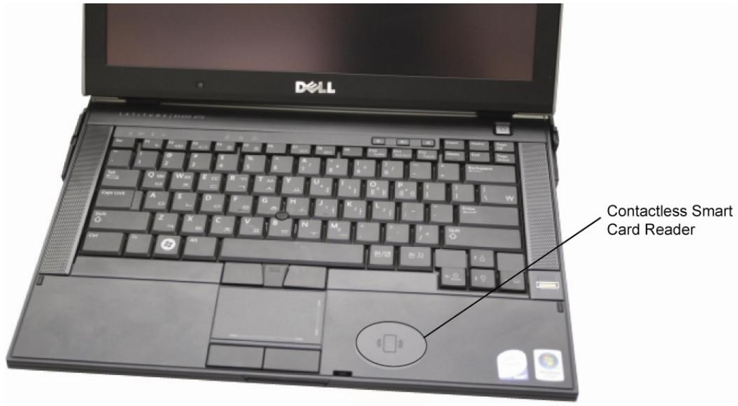
**Figure 5-1 Contactless Smartcard Reader Location**
