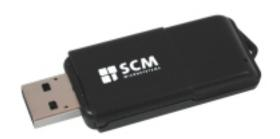
The SCL3711 from Identiv is as 13.56MHz USB NFC contactless smartcard reader supporting MIFARE and ISO 14443 A/B cards as well as Felica and all 4 types of NFC cards and tags in all 3 NFC modes (reader, card emulation and peer-to-peer). The reader is PC/SC compliant and comes complete with WHQL approved drivers for Windows and support for MacOS and Linux.
