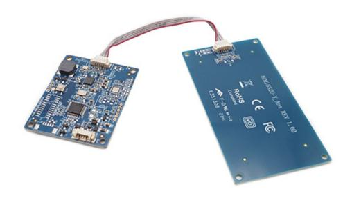
The ACM1552U-Y3 contactless and NFC reader module from ACS is a 13.56 MHz USB NFC solution that supports a wide range of technologies including NFC (card reader/writer, card emulation, and keyboard emulation mode), ISO 14443, ISO 15693, ISO 18092 and FeliCa devices.
