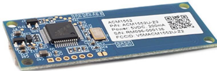
The ACM1552U-Z2 contactless and NFC reader module from ACS is a 13.56 MHz USB NFC module designed to be integrated into embedded systems. This reader module supports a wide range of protocols and technologies including NFC (card reader/writer, card emulation, and keyboard emulation), ISO 14443, ISO 15693, ISO 18092 and FeliCa.
