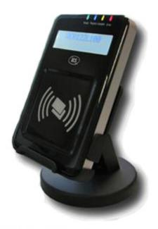
The ACR1222L USB desktop reader with LCD is an NFC contactless smartcard reader that has been developed based on the 13.56 MHz Contactless (RFID) Technology and the ISO/IEC 18092 Standard for Near Field Communication (NFC), supporting both NFC and Felica contactless technologies as well as MIFARE and ISO 14443 Type A and B cards. The ACR1222L is a USB Plug and Play device which allows interoperability with various different devices and applications.
