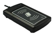
The ACR1281U-C2 from ACS is a 13.56MHz contactless reader device that appears to the host device/PC as a keyboard, and automatically reads the chip serial number (CSN) of each card when presented.
