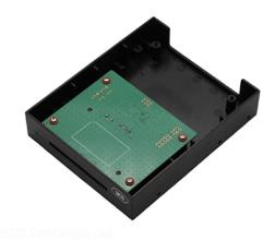
The ACR39F USB reader from ACS is based on the popular ACR39 electronics, housed in a lightweight frame that fits comfortably into a standard PC 3.5" drive bay. This reader is fully PC/SC, CCID and EMV Level 1 compliant and supports all ISO 7816 microprocessor-based smartcards as well as many popular memory cards.
