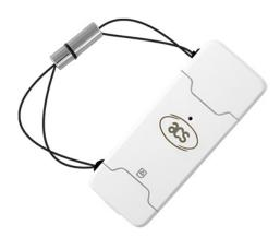
The ACR40T-A7 is a SIM-sized USB-C smartcard reader that features sophisticated technology and modern, compact design. The ACR40T-A7 supports ISO 7816, various memory cards and a wide range of T=0, T=1 microprocessor cards. This reader is functionally identical to the ACR40T-A5, but includes a configurable button that can be used to confirm the physical presence of the user, to comply with certain security requirements.
