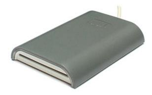
The Omnikey 5422 from HID is a dual interface USB smartcard reader that reads/writes to both 13.56 MHz contactless and virtually any contact smartcard technology.
