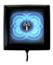
The DTAG100-NFC dynamic tag module from Dot Origin is a internal device that enables easy and rapid modification of NFC tag data via USB. Part of the well-established DTAG100 range of intelligent beacons and dynamic NFC tags, the DTAG100-NFC is designed to connect directly with digital signage, media players, PCs and other systems, offering complete platform independence without the need for software drivers or any knowledge of NFC protocols or tag data formats.
