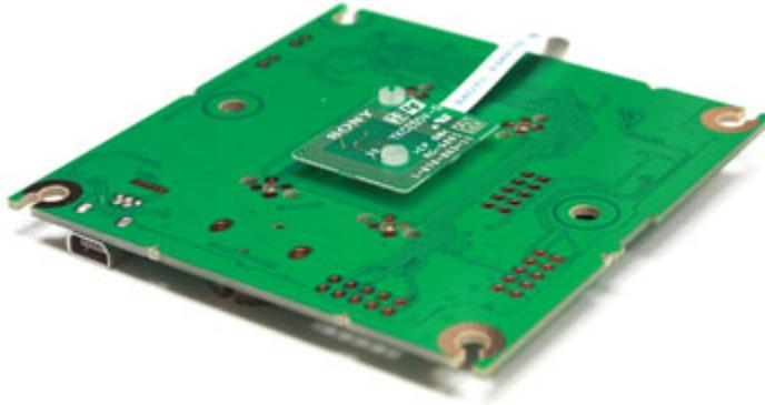
The DTAG100-NFC dynamic tag module from Dot Origin is an internal device that enables easy and rapid modification of NFC tag data via USB. Part of the well-established DTAG100 range of intelligent beacons and dynamic NFC tags, the DTAG100-NFC is designed to connect directly with digital signage, media players, PCs and other systems, offering complete platform independence without the need for software drivers or any knowledge of NFC protocols or tag data formats.
