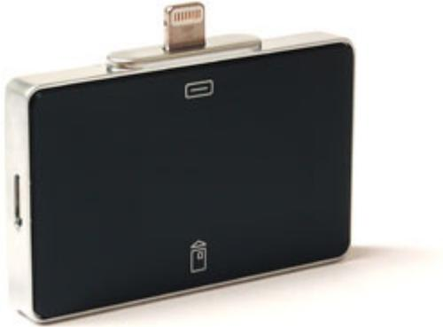
The iR301-L is a contact smartcard reader that enables smartcard applications to be deployed on iOS devices.
