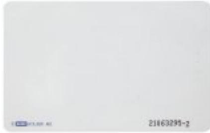
The iClass 2k/2 + Prox card from HID is a 13.56 MHz contactless smartcard designed for use with HID's door access control systems plus other compatible applications. The card also incorporates HID's 125 KHz Prox technology for migration from legacy systems. The iClass component contains 2k bits (256 bytes) of memory and is configured with 2 application areas. The first area stores the HID card number and the other is customisable for user requirements.
