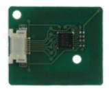
The FeliCa RC-S801 NFC Dynamic Tag from Sony is a 20 x 24mm contactless tag interface module that operates at 13.56 MHz in accordance with the NFC specifications. Rather than having any on-board data storage capabilities, it is designed to be integrated into other devices that can provide the tag data on each request, enabling it to return different responses each time it is read.
