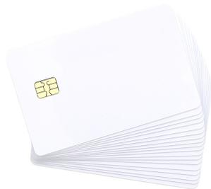
The SLE5542 is a standard, low-cost memory smartcard. It has 256 bytes EEPROM memory plus 32 x 1 bit protection memory. The SLE5542 is a fully-compatible, upgraded version of the SLE4442. Infineon has migrated the data carrier family to the IMEM CMOS technology. IMEM is conceived for security applications and offers unsurpassed physical and electrical protection schemes.
