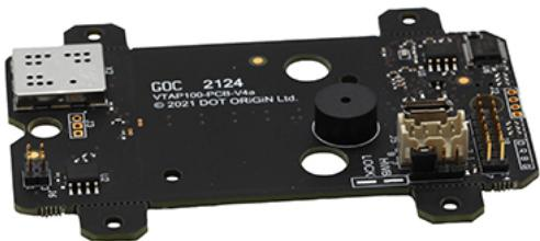
The VTAP100 from Dot Origin can selectively read and decrypt NFC pass data from iPhone or Android devices, and transfer this data to a connected system. It can also read unique IDs and secure encoded data from many RFID and NFC cards and tags, including MIFARE Classic and DESFire.
