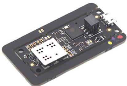
The VTAP50 from Dot Origin can selectively read and decrypt NFC pass data from iPhone or Android devices, and transfer this data to a connected system. It can also read unique IDs and secure encoded data from many RFID and NFC cards and tags, including MIFARE Classic and DESFire.
